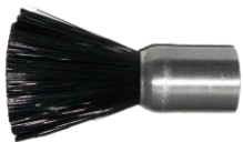
2049009 1/8BSP/F/P bristles 35 mm long 17 mm Ø overall length 60 mm
